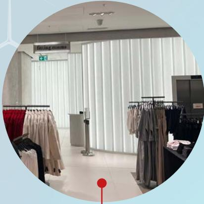
In the **LPP Reserved** stores, the Linit glass system is used to provide separation or screening between public areas and private areas. Linit Glass was installed on a tight curve and then backlit with strip LED lights to create bright feature walls which flow with the layout of the store.
